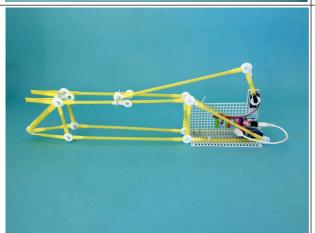
5. BUILD AND CONNECT THE SERVO ARM (10 min) We will now build the servo arm that controls the creatures movement. Connect the servo arm to adjustable connection on the back of the creature. Mind the servo arms start and stop positions and reposition the servo arm to make the movement suitable for the creature. Add a potentiometer if you need a smaller movement of the servo.
