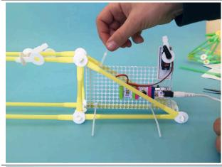
4. CONNECT LITTLEBITS TO CONSTRUCTION (10 min) Now it's time to connect the LittleBits to your creature. Use cable ties to secure the LittleBits build platform to the creature base.
